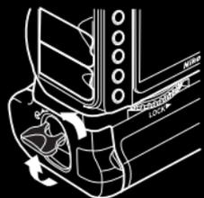
1. Ensure that the power is turned off on the camera and the Control Lock on the battery grip is in the "L" position. Turn the battery-chamber latch counter-clockwise to open the battery chamber door.
