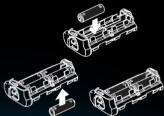
4. For AA batteries: Place six AA batteries of the same type in the AA battery holder, while ensuring that they are in the correct orientation. Mixing old and new batteries may cause accident.
