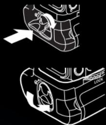
5. Insert the battery holder into the grip. Close the battery chamber and then turn the latch clockwise to lock. Turn on the camera and switch the control lock to be on "•" position and then check the battery level in the control panel or viewfinder.
