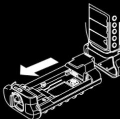
2. Remove the battery holder from the battery grip. The EN-EL15 Li-ion battery holder comes preinstalled when shipped.
