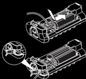
6. To use the DC adapter (sold separately): insert the adapter into the EN-EL15 battery holder in the same manner as a regular battery. Open the latch and pass the cable through.
