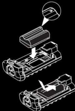
3. For EN-EL15 Li-ion batteries: Matching the indentations on the battery with the EN-EL15 holder, press the battery down and slide it in the direction of the arrow until the power terminals click into place.
