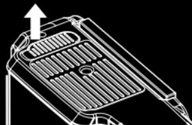
1. Please turn off the switch on the camera and ensure the control lock on the grip is in the "L" position before attaching.
