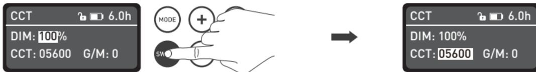
Press the SWITCH button to select from DIM, CCT and G/M.
