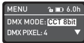
Press the SWITCH button to DMX MODE.
