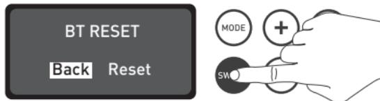
Press the SWITCH button to select Reset.
