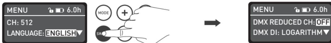
Press the SWITCH button to DMX REDUCED CHANNEL.
