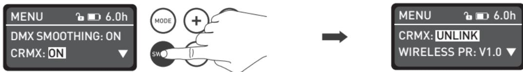
Press the SWITCH button to CRMX: UNLINK.
