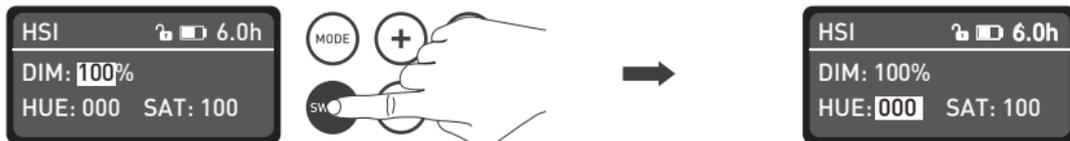
Press SWITCH button to select from DIM, HUE and SAT.
