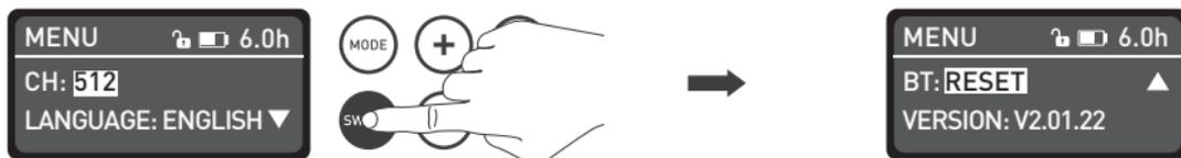
Press SWITCH button to VERSION to check the current version.
