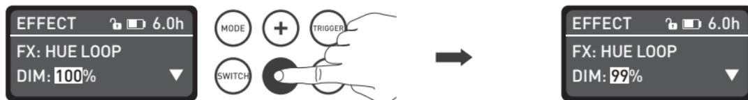
Press "+" or "-" to set the corresponding parameters.
