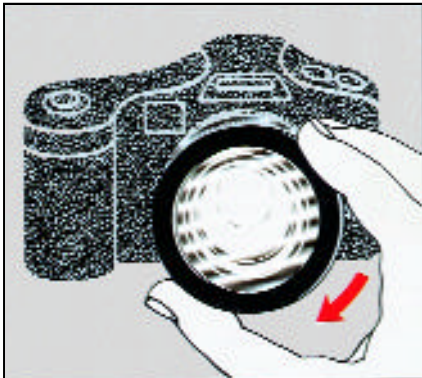
Screw the adaptor ring onto your lens.
