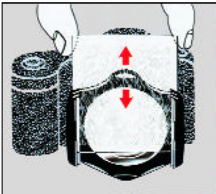
Slide the filter into one of the filter-holder slots.
