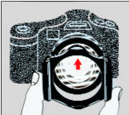
Slide the filter-holder on the adaptor ring until it snaps in place.
