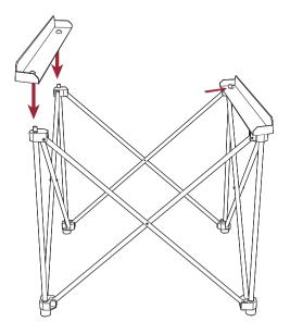
2. Attach the support rails onto the mounting posts, and slide to lock in place.
