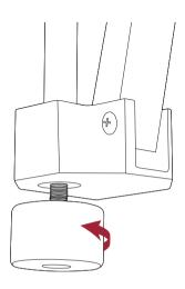
4. To level out the platform on uneven ground, rotate the leveling foot.
