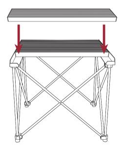
3. Seat the platforms onto the support rails.
