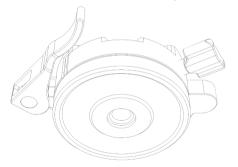
Remove the Quick Release Plate from the head by flipping the lever lock clamp to a 90-degree angle.
