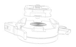
Insert Arca Swiss dovetail within the rails of the Arca Swiss clamping jaw.
