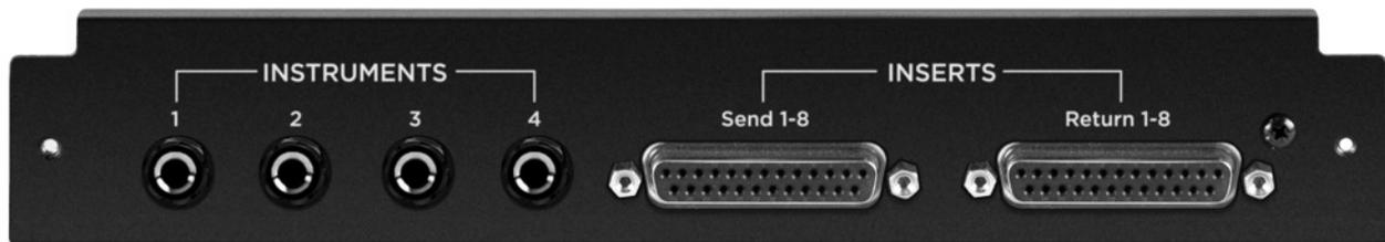
The Mic Preamp Module upgrades the functionality of any 8x8 or 16x16 module by adding mic preamps to the existing line inputs. A direct connection between the Mic Preamp Module and the Analog I/O Module inserts a mic preamp stage before the line inputs.
