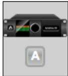
A device icon and ID button is placed adjacent to each row of parameters to identify the hardware unit to which the row belongs. By clicking on the ID button, the corresponding hardware unit's front panel will illuminate. Each hardware unit is assigned a Peripheral Prefix (A-Z, found in Maestro's Device Settings tab window) which is displayed on the ID button.
