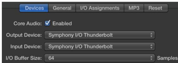
3. Start by setting the I/O Buffer Size to “64 Samples”. This setting may need to be adjusted based on your computer’s performance.
