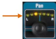
Touch the **Update** button. The update will start immediately. The screen goes blank and the Pan control indicators flash in sequence while the update is running. After a while the mixer will reboot.
