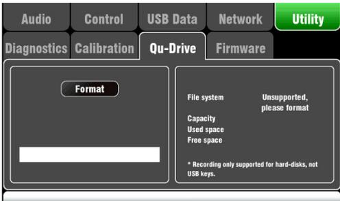
This screen lets you check and format a USB device (key or hard drive) for use with Qu-Drive. Once formatted you do not need to format it again.
