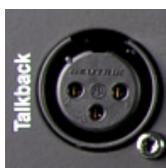
**Talkback Input** – Dedicated balanced XLR input for plugging in a microphone to route to the mixes for the engineer to talk to the performers on stage. Phantom power can be switched to the socket for condenser microphones.
