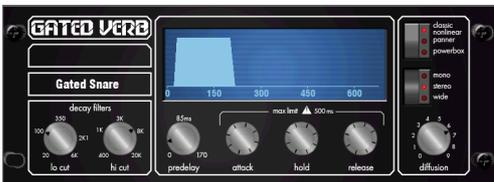
**Gated Verb** - An accurate emulation of the popular 80's Gated Reverb plus two other variants called 'Panned' and 'Powerbox'. The user interface gives instant access to Lo-cut Hi-cut decay spectrum filters and the gate envelope controls - pre-delay, attack, hold and release.
