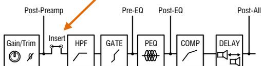
**Delay** up to 85ms can be added to each input channel. In most cases delay is not needed, but can be useful in time aligning sound from the PA to the acoustic sound from an instrument on stage. Allow 1ms per foot distance as a starting point.
