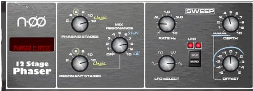
**Phaser** - A classic 12 stage emulation producing rich textured phasing with plenty of control. You can control the number of stages, feed forward and feedback, and 'zero' depth manual mode to manually sweep the Phaser using the offset control.
