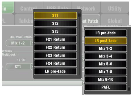
**Multitrack Playback** – You can play back your multitrack recordings from the hard drive plugged into the Qu-Drive port:
