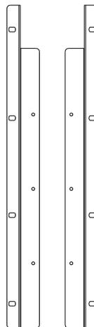
**Rack Mount Option** – A kit of parts is available from Allen & Heath to mount the Qu-16 in a standard 19" equipment case.
