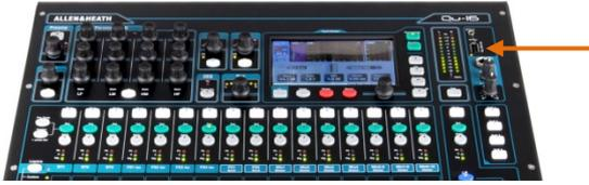
The Qu mixer operating firmware can be easily updated using a USB device (key or drive).
