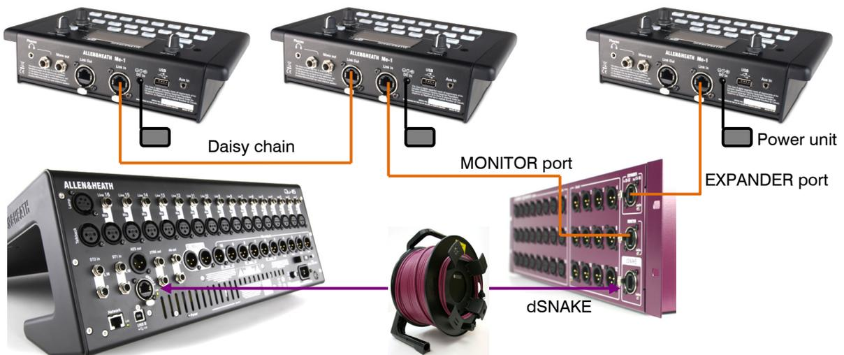
**Connecting ME to the Qu-16** - ME-1 mixers, a standard Ethernet switch or the ME-U hub can be plugged directly into the Qu-16 dSNAKE port if you are not using this to connect to an AudioRack. Power can be provided over the Cat5 by the ME-U or a PoE switch.
