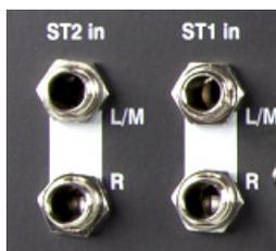
**Stereo Line Input** – ST1 and ST2 balanced 1/4" TRS (Tip, Ring, Sleeve) jack inputs for plugging in line level stereo sources such as CD players. The L input normals (switches) through the R input so that you can work with a mono source by plugging into just the L/M input.
