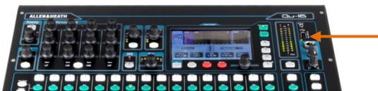
Plug in the USB device. Wait for the mixer to read the drive. The status window displays information about the USB device:
