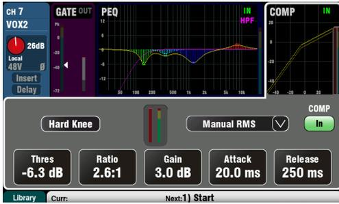
The Compressor is a powerful tool for controlling the dynamics of the sound, for example to smooth out a bass guitar or to narrow the dynamic range of a vocal to make it more intelligible in a busy mix. At its extreme setting the compressor can be used as a limiter to prevent the signal exceeding a preset maximum level.
