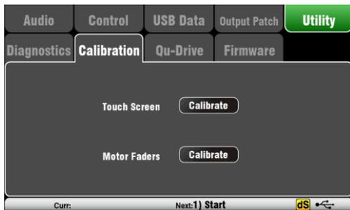
Use the routines here to calibrate the touch accuracy of the **Touch Screen** and positional accuracy of the **Motor Faders**.
