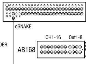
**Qu-24+2x AB168** – Expands with a second stage box to access all inputs.
