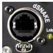
**Connecting Qu to the AudioRack** – Plug one end of your Cat5 'digital snake' into the Qu mixer dSNAKE port. Plug the other end into the dSNAKE port of the AudioRack.
