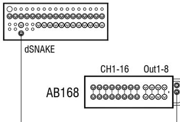
**Qu-16+2x AB168** – A second stage box expands the first to access ST1-3 on its first 6 inputs and provides more outputs. Inputs 7-16 are not used.
