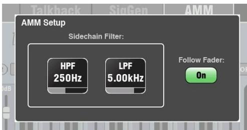
**AMM Setup** - Set High Pass and Low Pass filters for the input open mic detection to cut off frequencies below and above the normal speech range that may cause false triggering of the mics. Choose whether you want the signal used by the mix calculation to be affected by fader position.
