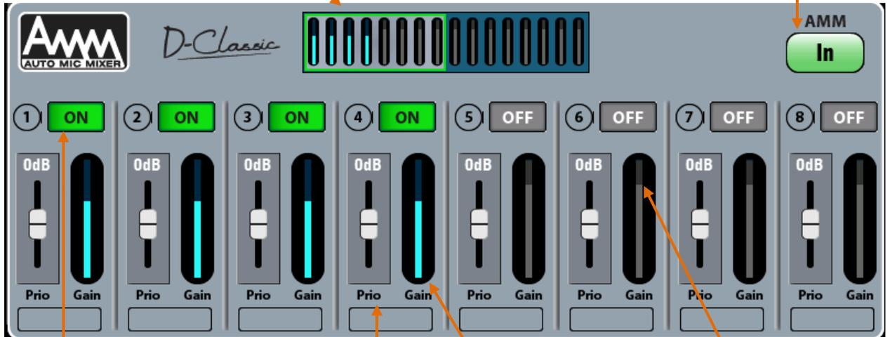
**ON/OFF** – Touch to turn on the channels you want to be affected by the AMM. The AMM sets the channel fader to '0', takes over gain control and lights the gain meter.
