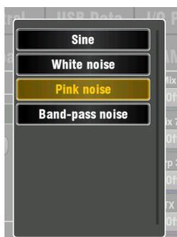
Set up and assign the Signal Generator to test loudspeakers and align levels between equipment.
