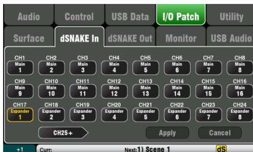
Use this screen to patch AudioRack input sockets to the Qu input channels. You can connect up to two AudioRacks via the dSNAKE Cat5 digital snake.
