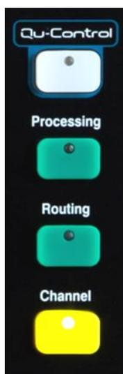
**Qu-Control** - User assignable custom screen for simple level, mute and on/off control. A user permission can be set so that this is the only control available to the 'Basic User', for example bar staff control of zone music source and level at a venue.
