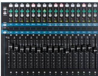
The Qu mixer has a group of fader strips, one per channel. These provide access to the input and master channel levels and processing.
