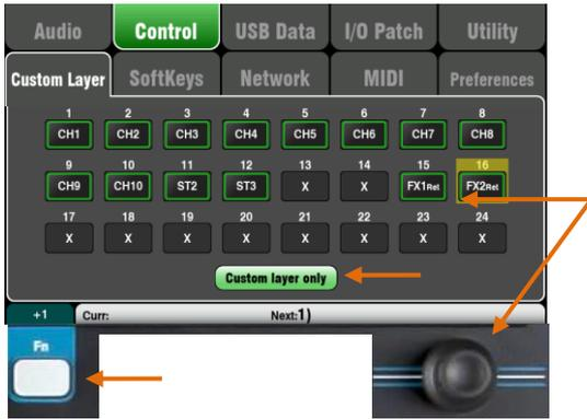
The Qu-16, Qu-24 and Qu-32 mixers provide a custom fader layer. The Qu-Pac does not have faders and provides a custom Select key layer (see below).
