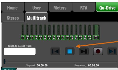
**Qu-Drive Multitrack page** – This screen presents the controls for multitrack recording to, and playback from a USB storage device plugged into the top panel Qu-Drive port.
