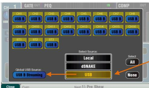
**Stream audio back to the Qu mixer** – Audio is returned via USB B. This is mapped one-to-one to the inputs channels. Use the **Preamp** screen **Fn** key Source page to patch USB B to the channels.
