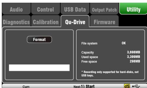
This screen lets you check and format a USB device (key or hard drive) for use with Qu-Drive. Once formatted you do not need to format it again.
