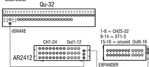
**ME Personal Mixing System** – The Qu system can interface directly or via the ME-U hub to ME-1 personal mixers using any available dSNAKE, EXPANDER or MONITOR port.
