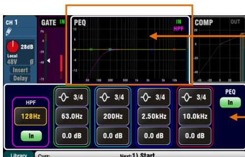
**Processing Screen** – When selected this screen presents the processing including Preamp, Gate, EQ, Compressor for the channel or master currently selected using its strip **Sel** key.
