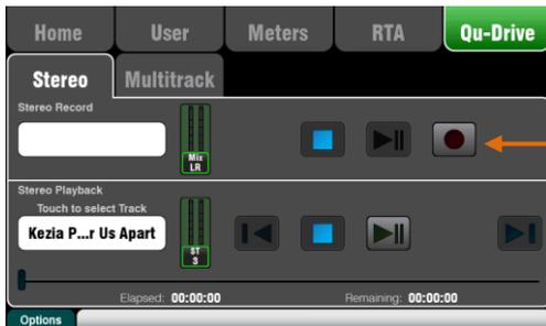
**Qu-Drive Stereo page** – This screen presents the controls for stereo recording to and playback from a USB device plugged into the top panel Qu-Drive port.
