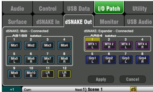
This screen presents the patching for the dSNAKE remote audio outputs. These outputs can be mapped from any combination of Qu mixer output sources.
