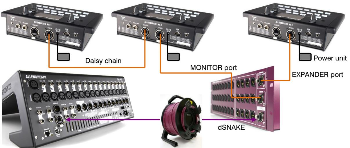
**Connecting ME to the Qu mixer** - ME-1 mixers, a standard Ethernet switch or the ME-U hub can be plugged directly into the Qu dSNAKE port if you are not using this to connect to an AudioRack. Power can be provided over the Cat5 by the ME-U or a PoE switch.
