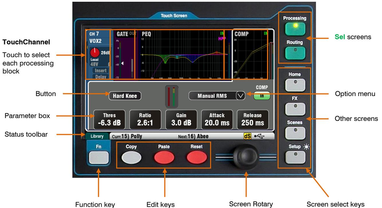
**Button** – Touch to select its function or change its state. Some functions need be touched for at least 1 second to avoid accidental operation, for example switching 48V phantom power or resetting the mixer. These are marked '(Hold)'.
