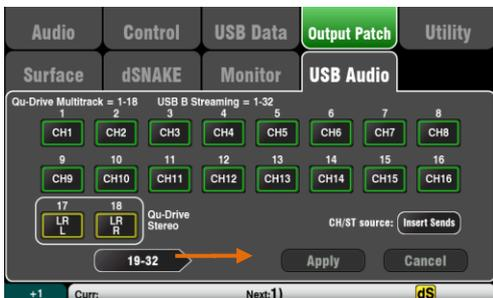
**Stream audio to the computer** – Audio is sent via the rear panel USB B port. Go to the **Setup / Output Patch / USB Audio** screen to choose which Qu outputs to patch to the USB stream.
