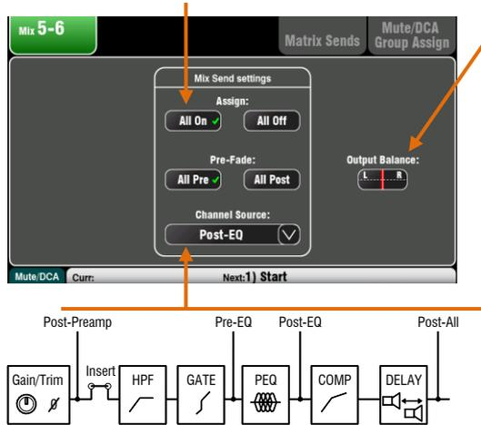
Select a mix master **Sel** key while the **Routing** screen is active to:
