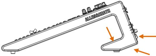
**Ventilation** - Make sure that air flow around the ventilation slots at the rear and underside of the mixer is not obstructed. Keep these areas clear when flight casing, installing or operating the mixer.
