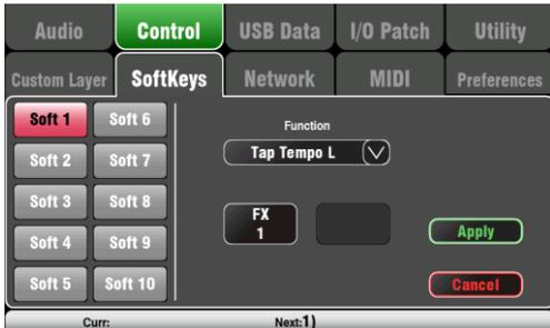
Qu-16 provides 4 SoftKeys. The Qu-24 and Qu-32 provide 10. Qu-Pac provides 15. These are called 'Soft' because they can be assigned to different functions by the user.
