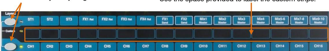
Turn on the **'Custom layer only'** option if you want to lock out the two standard layers and let the operator work with just the Custom layer.
