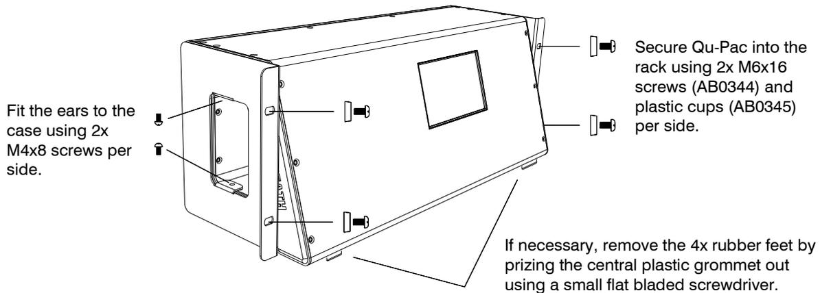
**i** Allow adequate air flow around the ventilation slots at the rear and through the inside section of the case. Do not block the sides.
