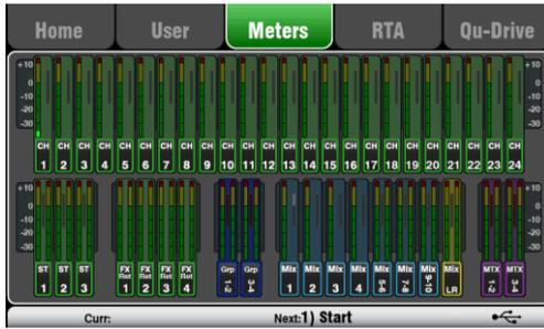
This screen provides a convenient view of all channel, mix and FX signal activity.
