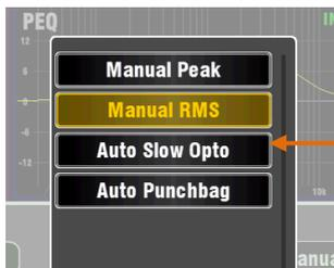
**Parameter box** – Touch to change its value. The box highlights orange to show it is selected and can be adjusted using the screen rotary.
