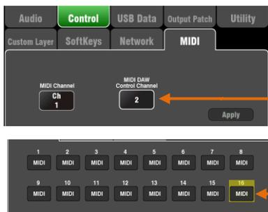
**Set the Qu mixer MIDI channel number** – Use the **Setup / Control / MIDI** screen to set the Qu MIDI channels. Qu DAW control uses its own MIDI channel. This is the next number up from that set for the other Qu MIDI messages. Qu defaults to Channel 1 for standard messages and Channel 2 for DAW control.
