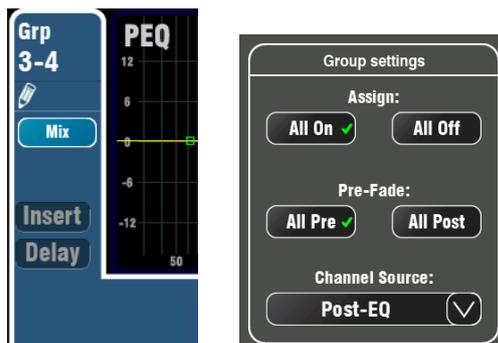
**Mix Mode** - Touch the **Mix** mode button to set operating mode as a stereo Mix. This provides channel send levels, dedicated pan, assignments, pre/post and source selection to the mix. You can assign combinations of channels, FX returns and groups to a mix. Mixes can be mixed to the Matrix.
