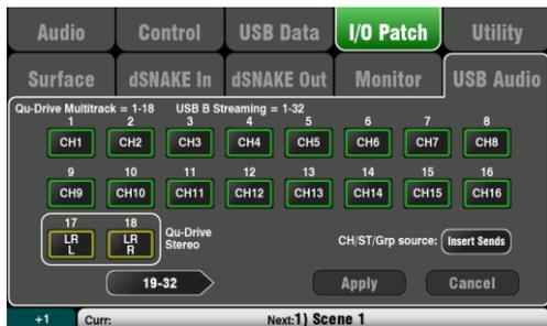
This screen presents the patching of the USB audio outputs. This includes the Qu-Drive Stereo, Qu-Drive Multitrack and the USB B audio streaming.
