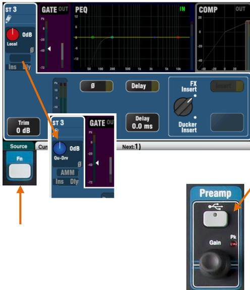
**Patch the playback to the ST3 channel** using the **Processing / Preamp** screen **Fn** key to open the Preamp Source screen. Make sure Qu-Drive is selected as the 'Global USB Source'. Select USB as the source for ST3.
