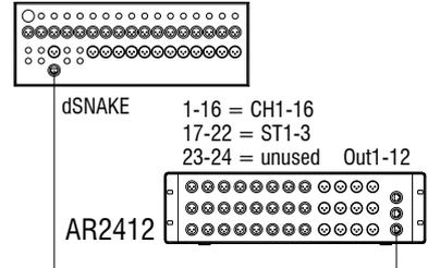
**Qu-16+AB168** – Provides a rugged digital snake and stage box for all 16 mic inputs and up to 8 returns.
