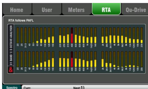
This screen displays a Real Time Analyser (RTA) which analyses the frequency content of the audio signal.
