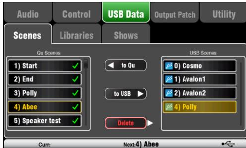
Individual Scenes can be transferred between Qu mixers via a USB device (key or drive) plugged into the Qu-Drive port. This provides a quick way to transfer settings without overwriting the current scenes and preferences.
