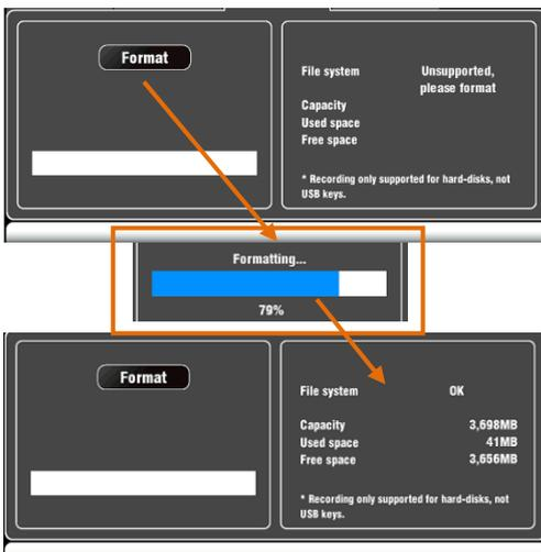
Plug in the USB device. Wait for the mixer to read the drive. The status window displays information about the USB device:
