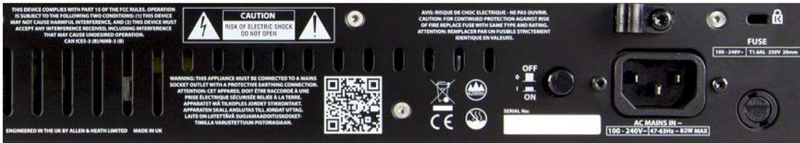
The Qu mixer has an internal universal voltage power supply unit. This means you can use your mixer in most parts of the world without the need to modify the unit as long the local mains supply is within the range:
