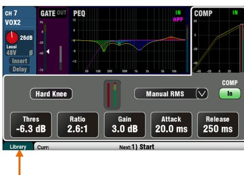
**Function Key** – The **Fn** key provides access to further options associated with the currently selected screen, for example channel source selection and processing libraries. It is also used to access the Mute Group and Matrix mix settings. If available, its function will appear in the lower toolbar above the key. Press the key again to close the option screen.
