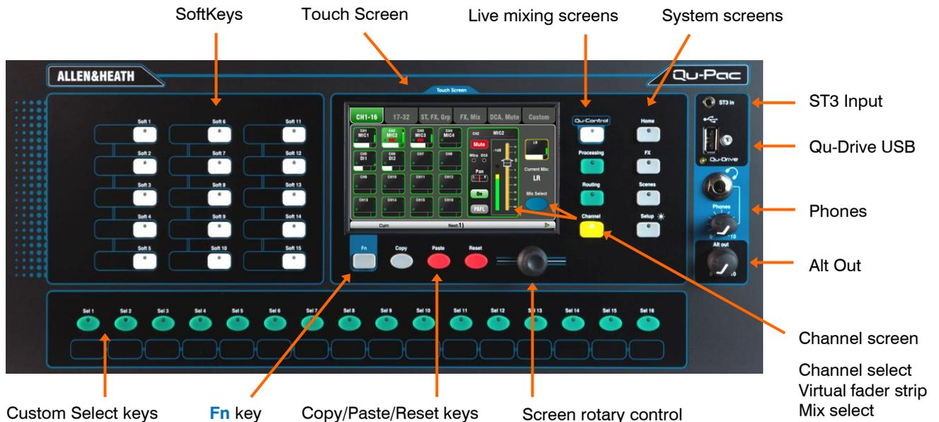
**Touch Screen** - All live mixing, setup and memory management functions can be controlled from the Qu-Pac front panel. The colour touch screen provides quick access to these functions. The top presents tabs for the available pages. The bottom presents a toolbar showing status information.
