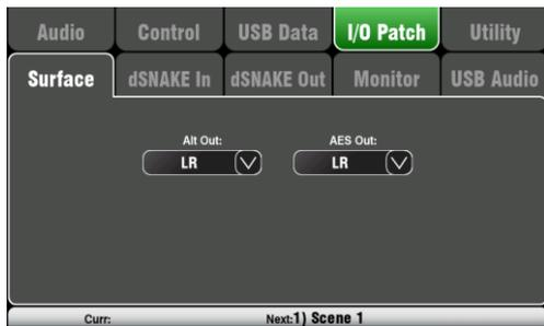
Use this screen to patch signals to the rear panel Alt Out and AES outputs. Touch a box to open up the list of available options. Changes are applied instantly. You can also touch outside the list to exit.
