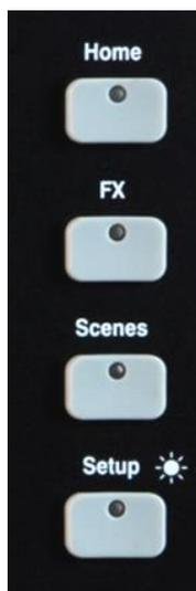
**Home** – Pages of housekeeping functions including safe Shut Down, Lock Surface, change and set up User Profile, view Meters and RTA, and work with Qu-Drive stereo and multitrack recording and playback.
