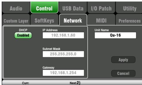
Use this screen set the TCP/IP address for the Network port and the name used to identify the Qu mixer on the network.
