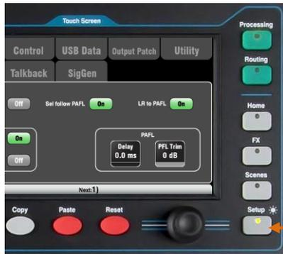
Touch the top tabs to access the different categories of setup function. Touch the tabs below to open up the related options available.
