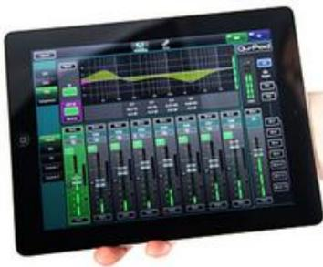
**Qu-Pad** is an engineer's mixing tool giving you the freedom to walk the room or stage and control the sound right where it is needed. Since V1.9, Qu-Pad gives you control of the live mix and full system setup. Qu-Pad and the Qu console can work together to provide simultaneous control of independent functions, for example one engineer using the console to mix front-of-house sound, and another using the iPad to mix monitors on stage.
