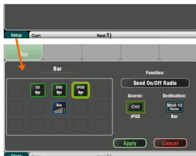
Functions can be assigned to up to 15 positions arranged as a grid of 3 rows with 5 columns. If a position is unassigned then it will appear blank in the user screen.
