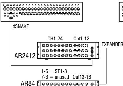
**Qu-24+AB168** – Digital snake for 16 mic inputs on stage.
