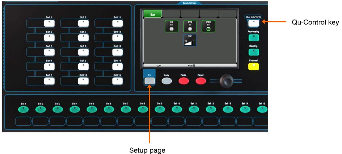
**Qu-Control key** - Press to open the Qu-Control screen. This presents buttons and level controls configured by the Admin user. If none have been configured the screen will be blank. Tabs allow access to up to 5 custom screens.
