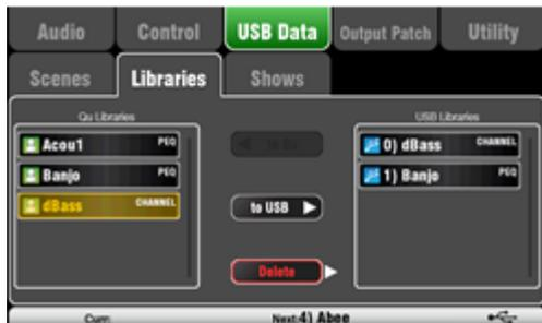
Individual processing and FX Libraries can be transferred between Qu mixers via a USB device (key or drive) plugged into the Qu-Drive port.
