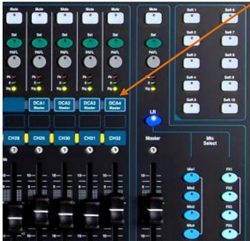
1. All Qu mixers provide DCA master controls in the **Routing** screen **Mute/DCA** view **Masters** tab. Press the **Fn** key to open this view.
