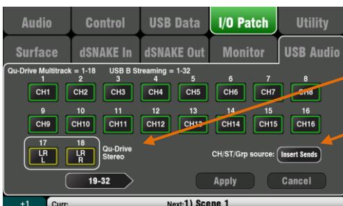
**Patch the source to be recorded** using the **Setup / Output Patch / USB Audio** screen. Touch the track 17 box and turn the rotary to select the left source. Press the '+ 1' **Fn** key to increment the right source to track 18, or use the rotary to select an unrelated source.
