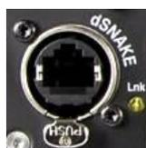
**dSNAKE** – The proprietary Allen & Heath ‘digital snake’ connection for remote audio using an AR2412, AR84 or AB168 AudioRacks, and for personal monitoring using the ME Personal Mixing System.
