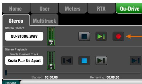
**Stereo Record** – You can record to a USB storage device plugged into Qu-Drive:
