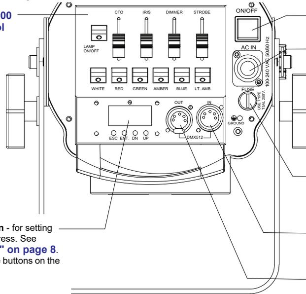
**Power Switch** - for turning fixture on and off.
