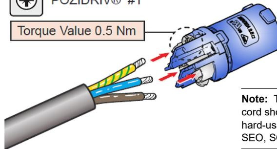
**Note:** The supply cord and connecting cord should be minimum 14AWG, extra-hard-usage types such as Type G, S, SE, SEO, SO, ST, STO, or W.
