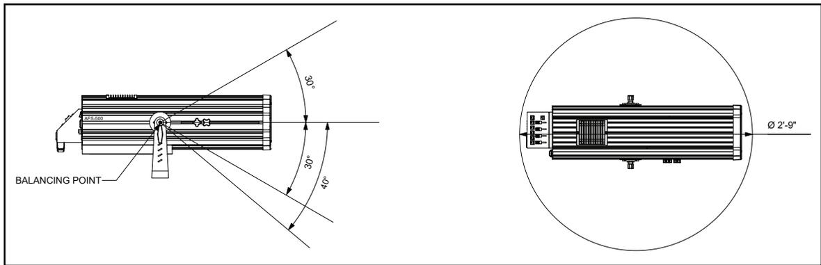
**Figure 2: AFS-500 LED Follow Spot Tripod / Fixture Movement**
