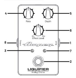
INPUT: The signal output from an instrument (active or passive) may be connected to this 1/4" Input by means of an unbalanced, (shielded) instrument cable.
