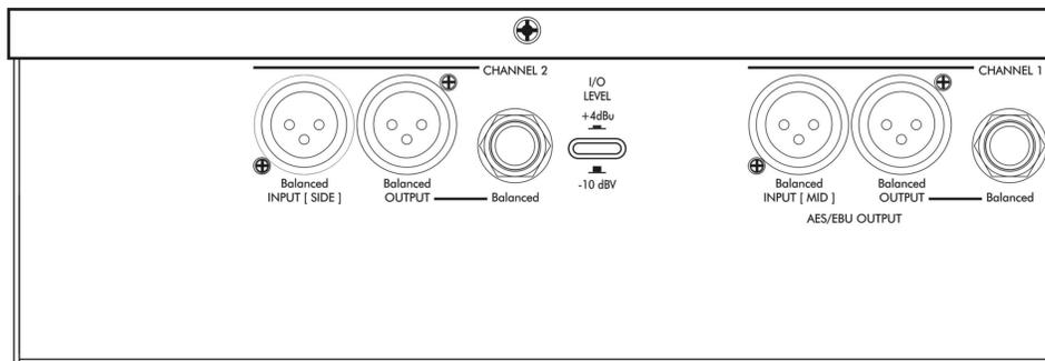
Figure 3 – Rear connections
