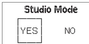
\*\* When Studio Mode is active, the light will turn on as soon as it receives power, without having to press the power button.
