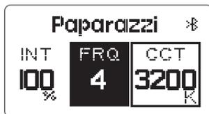
When in Lighting FX mode, rotate the CCT Control Wheel to adjust the base CCT of the lighting effect from 2700K to 6500K as displayed on the screen.
