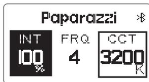
When in Lighting FX mode, short press the "Frequency" button to enter Frequency Adjustment Mode. Then rotate the Brightness Control Wheel to adjust the frequency of the effect from 1 to 10 and R (Random) as displayed on the screen.
