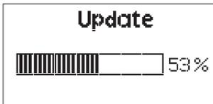
*\* Only FAT16 and FAT32 storage formats can be used for firmware updates. Incompatible formats will result in the screen displaying a format error and will return to the main menu.*
