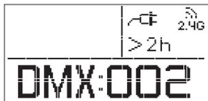
When in DMX mode, rotate the brightness control wheels to set the device's DMX channel. Then press the MENU button to take you back to the Menu interface.
