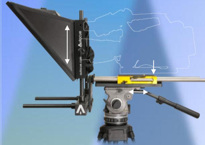
5. Mount the camera using the camera screw, access the screw from the under side of the plate (G). Please ensure that the lens is in the centre of the aperture on the back of the hood. To adjust the height of the hood loosen the tube clamps, adjust to the desired height and retighten to secure. The hood and bracket assembly can be moved forwards or backwards by loosening the rod adjustment clamp, once in the desired position retighten to secure.
