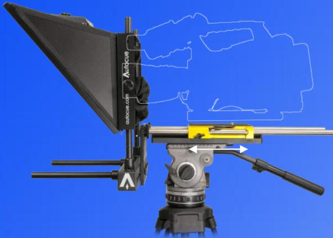
1. To balance the head with the camera mounted, slide the balance adjustment lever to the rear of the plate, the plate will now slide freely back and forth. When you have achieved a good balance slide the locking lever forward, this will lock the plate in this position.
