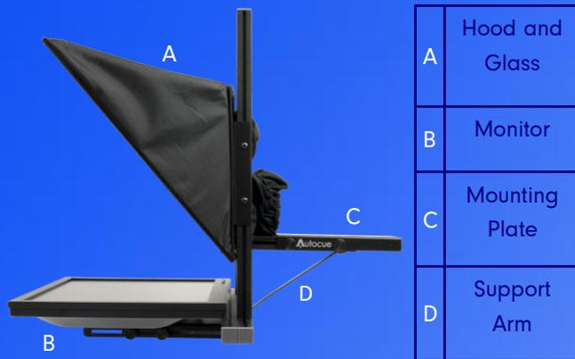
3. Attach the monitor to the hood mounting.
