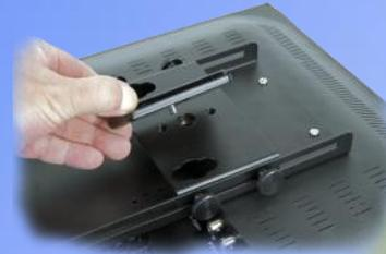
6. Secure the hot shoe in place using two screws if possible.
