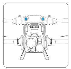
Fig 2-1 Front and rear visual lens modules of the aircraft
