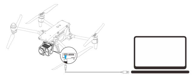
Fig 3-18 Connect to PC/MAC via Gimbal USB-C Interface
