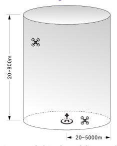
Fig 2-4 Diagram of altitude and distance limits
