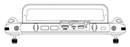
Fig 4-16 Custom Keys C1 and C2
