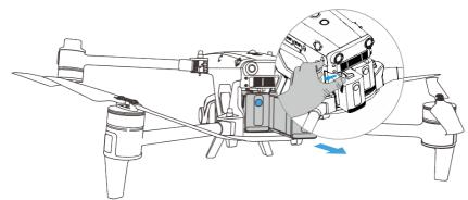
Fig 5-3 Remove the Smart Battery
