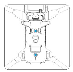
Fig 2-2 Upper left, upper right, and bottom visual lens modules of the aircraft
