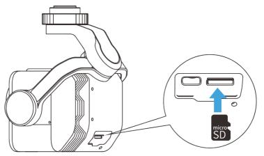
Fig 3-17 Installing the microSD Card
