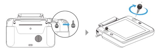
Fig 4-5 Installing command sticks
