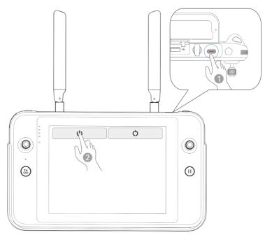
Fig 4-7 Turning the Remote Controller Off
