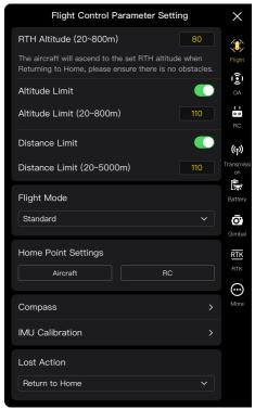
Fig 6-4 "Flight Control Parameter Setting" interface
