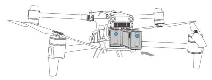
Fig 5-2 Install the Smart Battery
