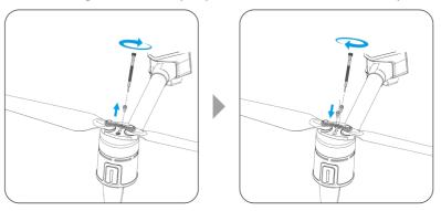
Fig 3-7 Install the Propellers
