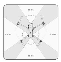
Fig 2-3 Observation Range of Millimeter-wave Radars
