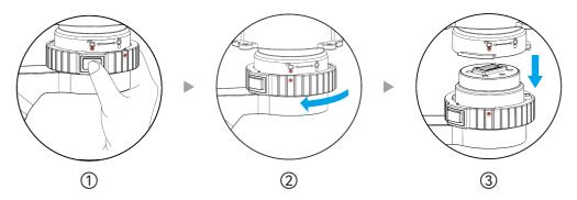
Fig 3-16 Removing the Gimbal
