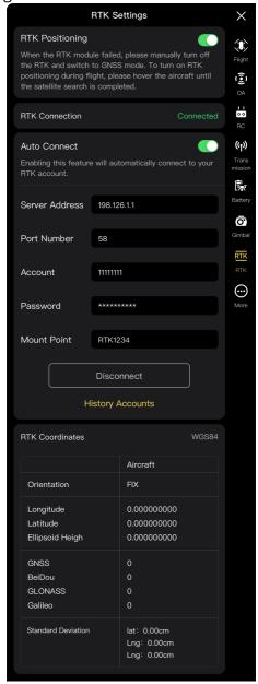
Fig 6-10 "RTK Settings" Interface
