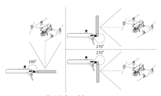
Fig 4-10 Extend the antenna
