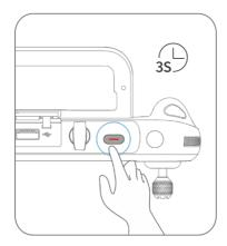
Fig 4-6 Turning the Remote Controller On
