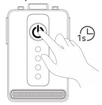
Fig 5-4 Checking Battery Level
