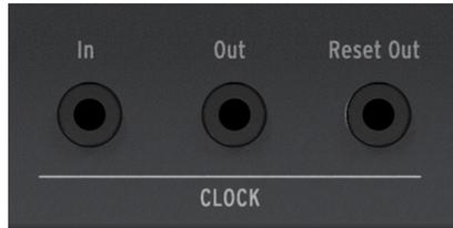
The KeyStep Pro is capable of both sending and receiving synchronization signals. It also has a Reset Out, allowing external sequencers with a reset input to re-start from the beginning of a sequence whenever a KeyStep Pro sequence is restarted.
