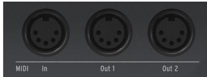
The KeyStep Pro can send not only MIDI note-related data but also MIDI synchronization signals, so that your external tempo-dependent devices (such as sequencers, arpeggiators, etc.) remain in sync.
