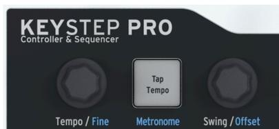
The Tempo/Fine knob sets the tempo from 30-240 beats per minute (BPM). As you turn this knob, the BPM value is automatically rounded off to the nearest whole number and shown on the KeyStep Pro's OLED display. Holding down 'Shift' while turning this knob gives you finer BPM control by switching off the whole-number rounding.
