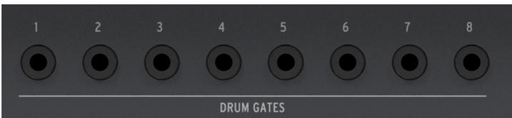
**i** ℹ: These gate signals are not limited to triggering drum sounds. You can connect these outputs to any input that accepts a trigger or gate signal, including an ADSR envelope generator or an LFO reset. Experiment, and we're sure you'll find some delightful rhythmic uses!
