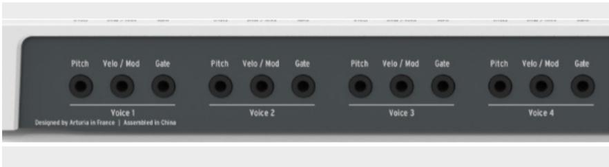
The Pitch CV output is mostly used to control the pitch of an external voltage-controlled oscillator (VCO).
