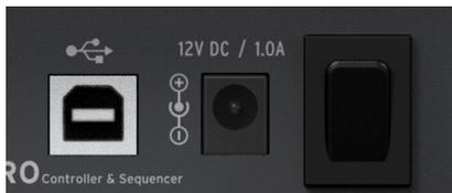
The USB connector provides a data connection to your computer or tablet for those occasions when you want to use the KeyStep Pro with a host device. When working this way, simply connect the KeyStep Pro to your host device with the supplied USB cable and switch it on.
