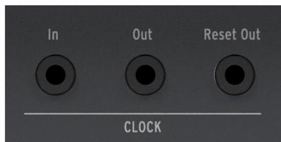
The ON cycle of the Clock output (Clock Out) is +5V, which should be enough to trigger even the most unresponsive Eurorack modules.
