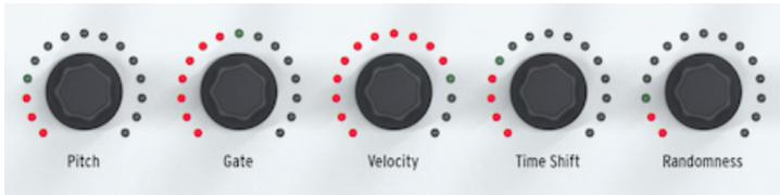
Each of the five main encoders is surrounded by 15 red LEDs, each of which has eight levels of brightness from dim red to bright red. If we take the Gate encoder as an example: first turn it all the way counterclockwise, then turn it slowly to the right. The LED in the first position will slowly increase in brightness and after eight clicks the second LED will light up dimly and the dim-to-bright cycle will repeat. All in all, this gives you 128 distinct positions for each of these encoders!
