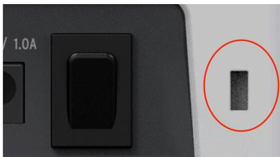
We've included a Kensington lock slot on the far right edge of the back panel so you can secure it to the surface of your choice.
