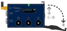
Insert battery with key on lower side.
