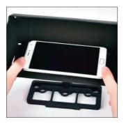
Tighten the thumbscrew of the holder to eliminate movement while handling the remote.
