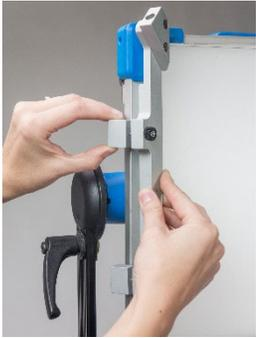
With the pole holes pointed outward from the fixture slide the metal bracket over the front of extrusion on the SkyPanel. This should hook in between the front of the fixture, and the metal extrusion. The metal blocks will then hook around the rear of the extrusion. Tighten the thumbscrews, ensuring the bracket is secure.
