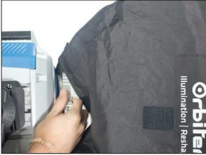
Once the Lightbank body is set up on the Speed Ring, attach your Chimera Lightbank for ARRI Orbiter to fixture via the Quick Lighting Mount. Rotate clockwise until you hear a click.
