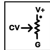
Do not use any other ground source. If multiple remote DC level controls are used for different channels, the same ground and V+ sources can be shared.
