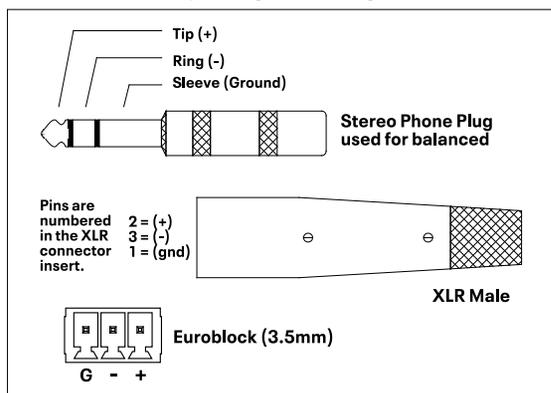
Each channel's Euroblock, 1/4" phone jack, and XLR inputs are wired in parallel, with XLR pin 2 (+) and pin 3 (-). When using an unbalanced input, wire the signal to the input (+) Euroblock pin, phone jack tip, or XLR pin 2, and also be sure to wire the input (-) pin, phone jack ring, or XLR pin 3 to ground. Do not leave the (-) input unconnected. Avoid running low
