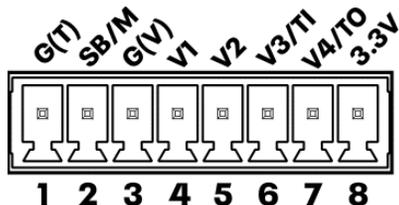
Some GPIO pins have multiple functions depending on their configuration. Each pin function is described below, as well as in the Settings>GPIO configuration menu.
