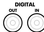
A S/PDIF digital audio output jack is also fitted. The S/PDIF output signal by default reflects the input to amplifier installation zones A & B and is intended to be used for daisy chaining FX amplifiers.
