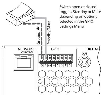
Diagram 7.1: GPIO Connections for remote standby/mute switch
