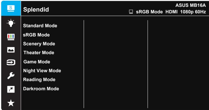
1. Press the Central of 5-way button
