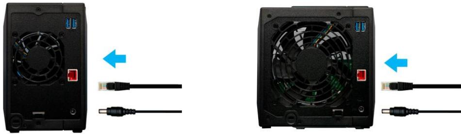
2. Connect the NAS to your router, switch or hub using an Ethernet cable.
