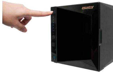
4. The NAS is ready for operation once the green system status LED indicator has stopped flashing and remains steadily lit. At this time, you should also hear a 'beep' from the system buzzer. Hardware installation is now complete. Please move on to the software installation guide to configure your system settings.
