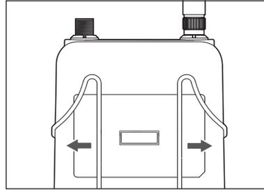
Pull both sides of the clip firmly to the outside to remove the clip from the transmitter.
