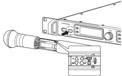
3. Press the SYNC button on the transmitter.
