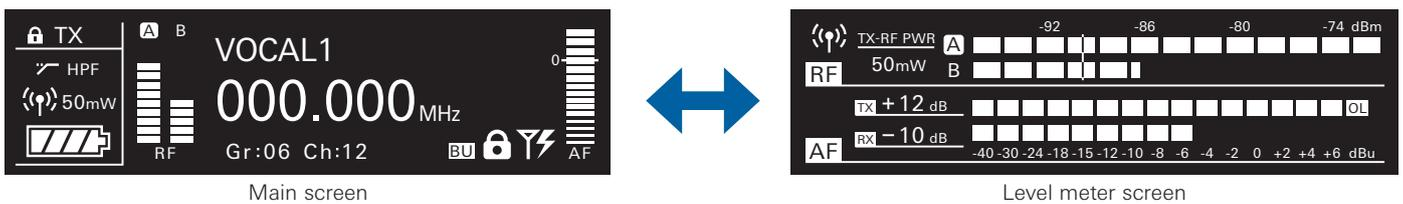
The main screen is switched every time the function button 2 is pressed.
