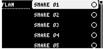
As with probability the amount of flam is set using the tap button and rate control, and its level of use is set in preferences. The flam sub-menu allows it to be selected on a drum-by-drum, step-by-step basis. **Note Repeat**
