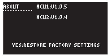
The About sub-menu shows the current firmware version for each of the two MCUs and allows a restoration of factory settings using the Yes button (33). Note that factory restore will wipe out any programming, so please back up your work either to SynthTribe or a SysEx app such as MIDI  $OX^{TM}$  for Windows, SysEx Librarian for Mac OS.
