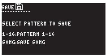
This button is used to save the current pattern or song. Follow the instructions on the display to action.4444 Pressing the pattern button while in save mode allows any of the sixteen patterns associated with the current song to be saved. Pressing the song button allows any of the eight songs in memory to be saved. The selection is made using the sixteen pad/step buttons. Press save again to confirm the save operation and exits the menu. **COPY**
