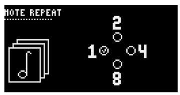
Step repeat is used to loop a number of steps. Use buttons 35 – 38 to select whether 1, 2, 4 or 8 steps will be repeated. Pressing the trigger button will cause that number of steps to repeat until the button is released. **NOTE REPEAT**
