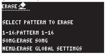
The erase button allows any pattern, song or global settings to be erased for memory. Pressing the pattern button while in erase mode allows any of the sixteen patterns associated with the current song to be selected to be erased. Pressing song allows any of the eight songs to be selected, using the sixteen step/pad buttons. Pressing menu selects all of the global settings. Pressing the erase button again confirms the erasure and exits the menu. **DUMP**
