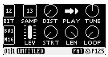
The default menu is that which shows on the display when none of the sub-menus accessed by the Menu button, as described below, is in use. It shows the settings of various parameters and alters when they are changed. Some parameters can only be selected for editing in this screen, some can be edited in this or the second screen. When a parameter is changed the changes are automatically saved. Edits are non-destructive, so making further adjustments is possible. **TOP ROW**(left to right)
