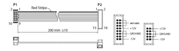
Connect end P1 to the module socket Connect end P1 to the module socket
