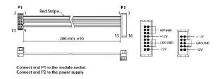
The module comes with the required power cable for connecting to a standard Eurorack power supply system. Follow these steps to connect power to the module. It is easier to make these connections before the module has been mounted into a rack case.
