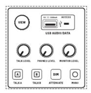
A USB type-A connector allows a flash drive to be plugged directly into the console for saving or loading data. This allows you to back up your show files or load your usual setup on a rented WING console.
