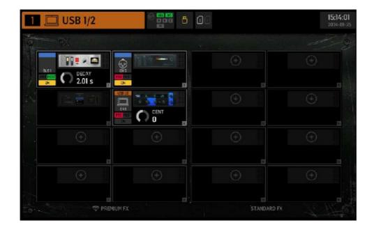
The EFFECTS screen controls all aspects of the effect processors. Users can select from a large collection of virtual emulation of analog processors, configure routing, adjust parameters and monitor levels.
