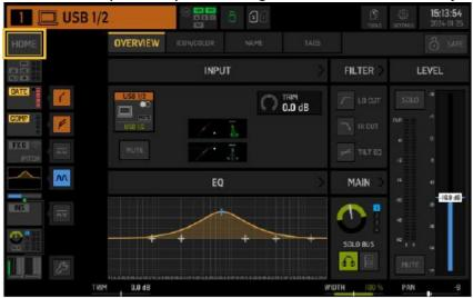
The processing sequence of the gate, dynamics, EQ, and insert sections, as well as the tap point for the signal sent to the 16 buses can be adjusted by clicking on the wrench icon on the bottom-left corner of the HOME screen and dragging the blocks.
