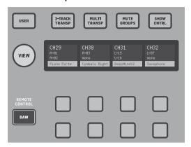
The bottom portion of the Custom Control section allows quick access to different categories. Press the VIEW button to configure each of them. It offers a combination of user-assignable buttons and pre-configured buttons for controlling the USB recorder, the WING LIVE recorder, Mute Groups and Show Control.
