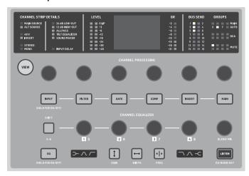
The channel strip provides quick access to the primary parameters for the currently-selected channel. A display screen provides dedicated editing details for the parameter being adjusted, and various indications for input configuration, bus and group assignments, and metering are always visible for convenience.
