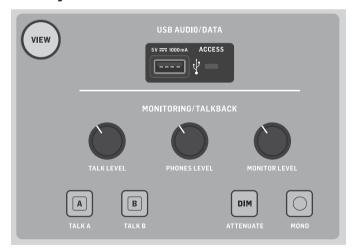
A USB type-A connector allows a flash drive to be plugged directly into the console for saving or loading data. This allows you to always have a backup of your show files, or even use a rented WING console while retaining your usual setup. The connector also allows recording and playback of audio files. The port can charge a portable device such as a phone or tablet, which is especially convenient if you frequently rely on a device like this to mix wirelessly.
