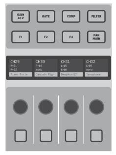
The edit section above the righthand fader bank offers a special set of dedicated control elements. This can be parameters like gain, pan, filters or effects sends for the selected bank of 4 channels.
