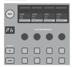
The Custom Controls section allows up to 4 rotary knobs and 8 buttons to be configured for control of specific elements that should be available at all times regardless of the main display screen focus. A common use could be the vocal channel's reverb send level. Presets can also be configured to suit different sets, venues, operators, etc. Press the VIEW button to assign functions to the controls, optimize the scribble strips, or reset the controls.
