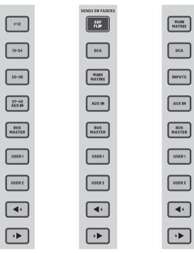
Selecting different fader banks will instantly bring a new set of channels to the associated fader section, including the scribble strip names/icons, and the motorized faders will jump to their correct positioning. If a particular bank does not fit on the available physical faders in a section (for example, Bus Masters), the shift arrows will scroll in blocks of 4 to access the remaining channels. Each fader section also has 2 user-defined banks that can contain a variety of channels.
