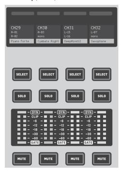
Each fader strip has a mini display screen called a scribble strip. This will indicate information about the current channel/bus number, name and even a graphic icon to quickly identify which channel is currently controlled by the fader and associated buttons. A color bar above the scribble strip allows quick visual identification of groups of related channels. Scribble strip details and color bar options can be edited on the HOME screen/HOME tab by pressing the CUSTOMIZE button.
