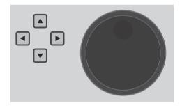
The navigation arrows and value/scrub wheel perform functions pertaining to DAW control as well as the USB Audio and WING-LIVE players. The wheel can also fine-tune values of parameters assigned in the User layer of the Custom Controls while respective buttons are depressed.
