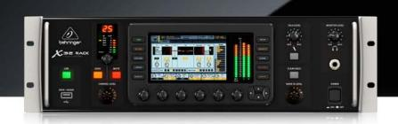
40-Input Channel, 25-Bus Digital Rack Mixer with 16 Programmable MIDASPreamps, FireWire\*/USB Audio Interface and iPad/iPhone\* Remote Control
