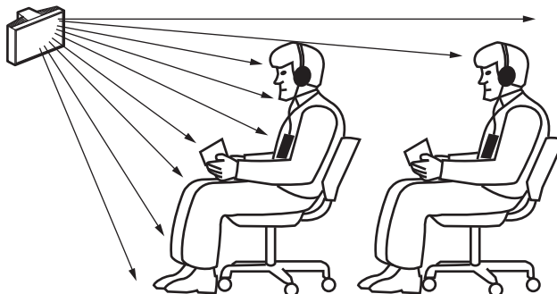
Figure 4.10: Infrared signal blocked by a person in front of the participant
