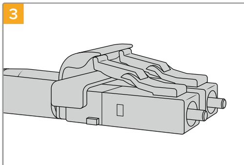
The optical fiber cables have latching tabs on top to make sure they don't fall out.
