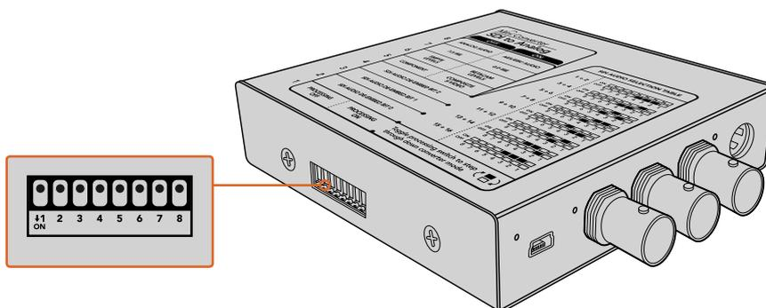
Change settings by adjusting the switches with a pen.
