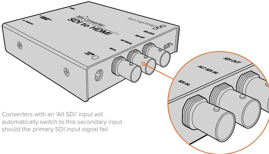
Converters with an 'Alt SDI' input will automatically switch to this secondary input should the primary SDI input signal fail.
