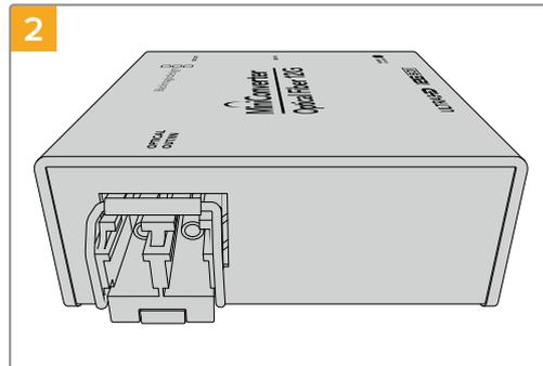
Remove the protective cover from the SFP optical fiber module, and insert it in the SFP socket. A locking pin clicks into position to secure the module in the socket.
