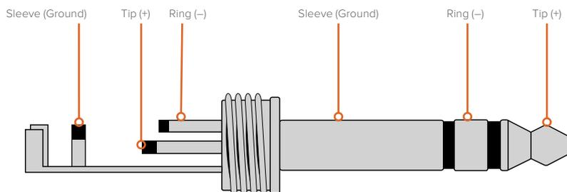
The audio jack illustration on the previous page shows the jack connector's positive, negative and ground wiring pins. If you need to reverse the polarity of your analog audio cable to suit your audio equipment, you can simply swap the positive and negative wiring on the tip and ring pins.
