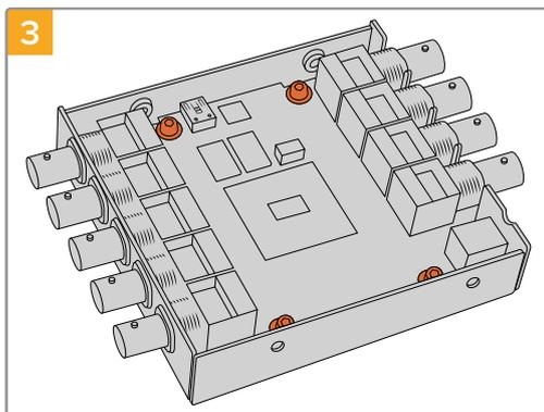
Using a T10 torx screwdriver, remove the four screws connecting the circuit board to Mini Converter SDI Distribution 4K’s frame.
