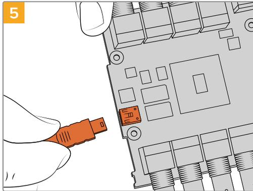
Plug in your Mini Converter SDI Distribution 4K's power supply and connect it to a computer using a USB cable. Update the internal software as you would any other mini converter.
