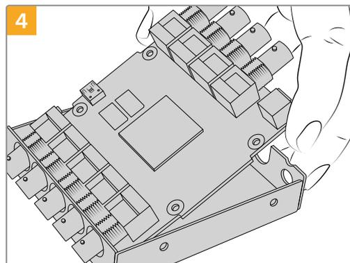
Gently pull the circuit board from the frame to access the USB connector.
