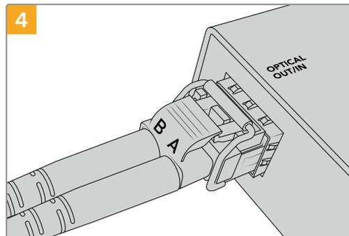
Plug in the optical fiber cables. Confirm the Out and In plugs are in the correct sockets, and that the locking tabs on the plugs hold the lever of the SFP optical fiber module upright.
