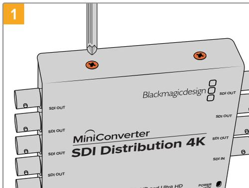
Using a philips head screwdriver, remove the four (M3) screws on the sides of Mini Converter SDI Distribution 4K.
