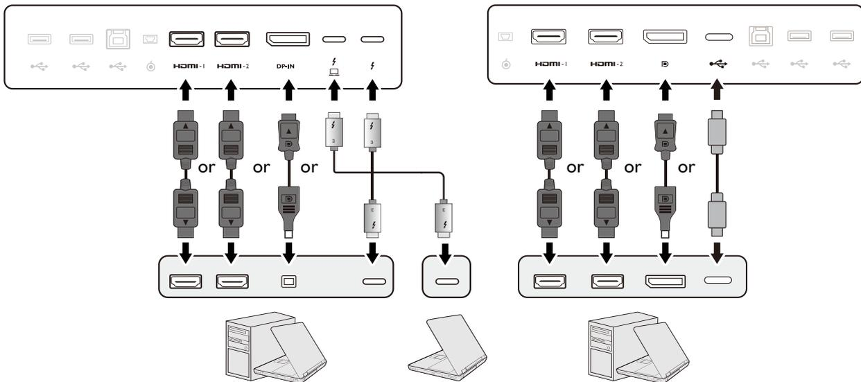
2. Connect the other end of the video cable to an appropriate port of a digital output source (e.g., a computer).
