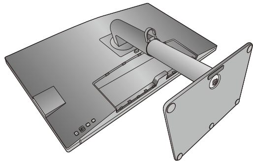
Use a cross-pointed screwdriver to release the screws that fixing the back cover to the monitor. The use of a magnetic-head screwdriver is recommended to avoid losing the screws.
