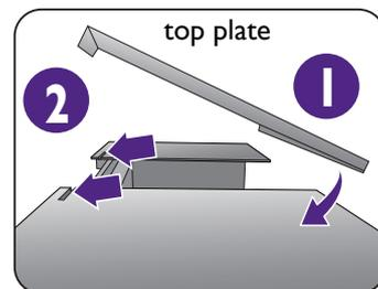
7. If you intend to calibrate the display's color by a colorimeter, slide to open the cover on the top plate so the colorimeter can be installed.
