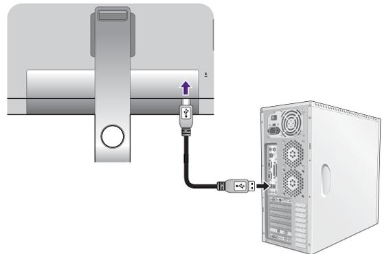
Connect USB devices via other USB ports (downstream) on the monitor. These downstream USB ports transmit data between connected USB devices and the upstream port.
