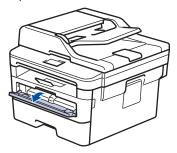
3. Use both hands to slide the manual feed slot paper guides to fit the width of the paper you are using.
