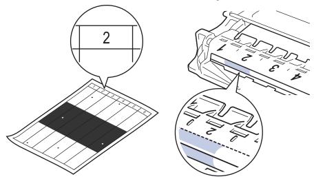
11. Turn the edge of the drum unit toward you while looking at the drum surface to find the mark.
