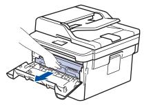
8. Push down the green lock lever and take the toner cartridge out of the drum unit.
