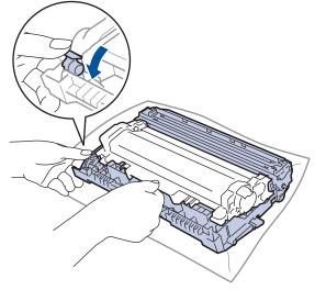
9. Turn the drum unit as shown in the illustration. Make sure that the drum unit gear is on the left side.
