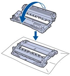
10. Use the numbered markers next to the drum roller to find the mark on the drum. For example, a dot in column 2 on the check sheet means that there is a mark in drum region "2".
