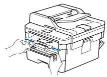
5. Using both hands, put one envelope in the manual feed slot until the front edge touches the paper feed roller. When you feel the machine pull it in, let go.
