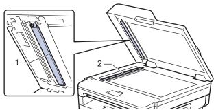
4. Open the scanner glass cover (1), and then clean the other white bar (2) and scanner glass strip (3) (supported models only).
