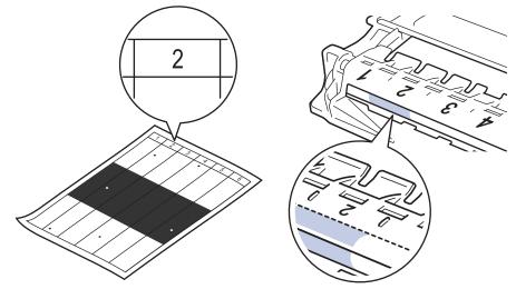
11. Turn the edge of the drum unit toward you while looking at the drum surface to find the mark.
