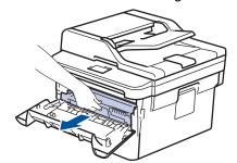
8. Push down the green lock lever and take the toner cartridge out of the drum unit.
