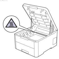
6. The color of printed dots on the Drum Dot Check Sheet is the color of the drum you should clean. Remove the toner cartridge and drum unit assembly that matches the color causing the problem.
