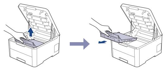
5. Remove the orange packing material and discard it.
