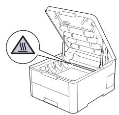
3. Remove the toner cartridge and drum unit assembly for the color shown on the LCD.
