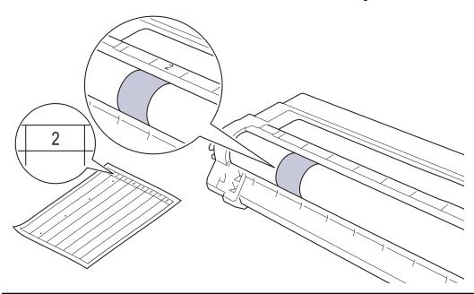
12. Wipe the surface of the drum gently with a dry cotton swab until the mark on the surface comes off.
