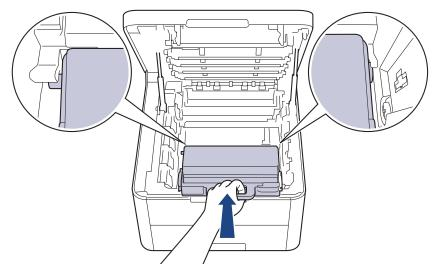
8. Reinsert the belt unit into the machine.
