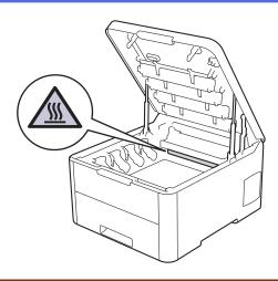
7. The color of printed dots on the Drum Dot Check Sheet is the color of the drum you should clean. Remove the toner cartridge and drum unit assembly that matches the color causing the problem.
