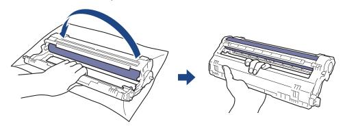
10. Loosen your grip so the frame drops forward, and then use your right hand to locate the drum unit gear inside the right side of the frame.
