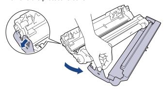
7. Reinsert the toner cartridge firmly into the new drum unit until you hear it lock into place.
