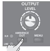
Each time you press the button, the setting alternates between XLR+LINE, XLR only, LINE only, and both off. The indicators light to indicate the jacks from which the ambience is output.
