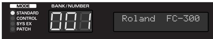
When the power is turned on, the FC-300 starts up in Standard Mode.
