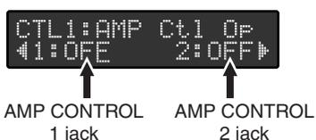
Control of AMP CONTROL using a pedal when the AMP Ctl Op parameter is set to ON and the AMP Pol. parameter (p. 50) is set to NORMAL is as shown below.
