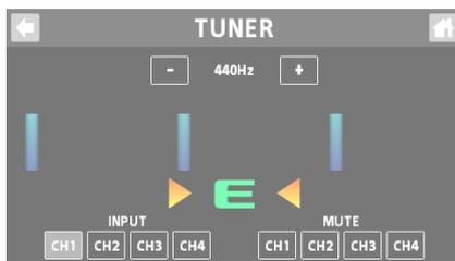
2. Touch INPUT <CH1>--<CH4> to select the channel used for tuning.
