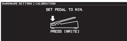
**2. Press the heel end of the pedal, and press the [WRITE] button.**
