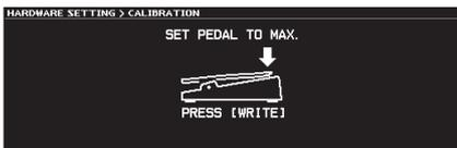
**3. Press the toe end of the pedal, and press the [WRITE] button.**
