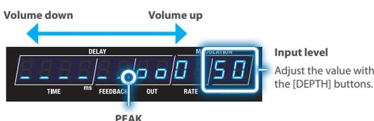
When the input signal exceeds this level, the sound begins to distort.
