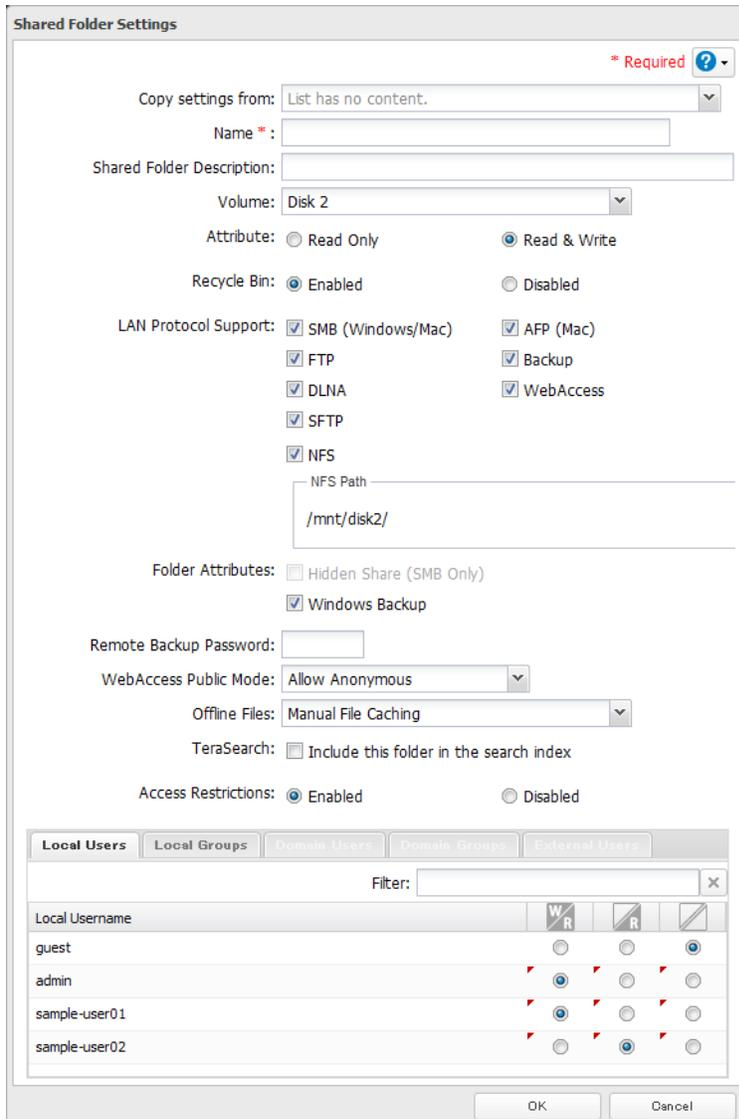
**Note:** To configure a password, enter it in the “Remote Backup Password” field. Leave this field blank if you don’t want a password. If the target device is configured with a backup password, you can easily find the backup target folder during configuration of the backup job by searching for the password.
