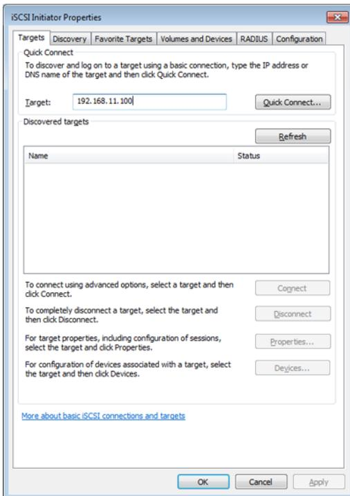
**13** The connected volume will be recognized by the computer as an unallocated volume. Assign and format the
