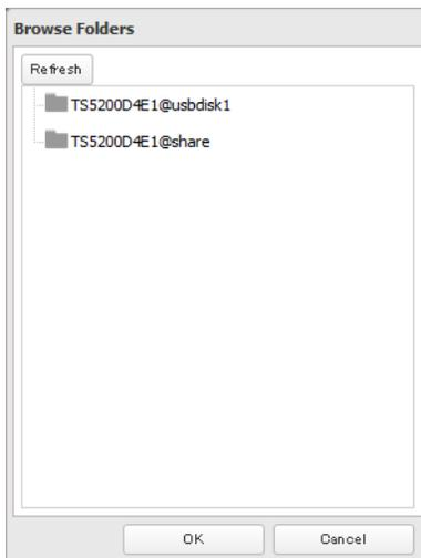
**Note:** If you will use the same folder for both Amazon S3 remote replication and as a backup target folder, create a new subfolder under “\wbfs\amazons3”. Under “LAN Protocol Support”, enable “Backup”. Without these settings, that shared folder will not be listed in the backup target folder list.
