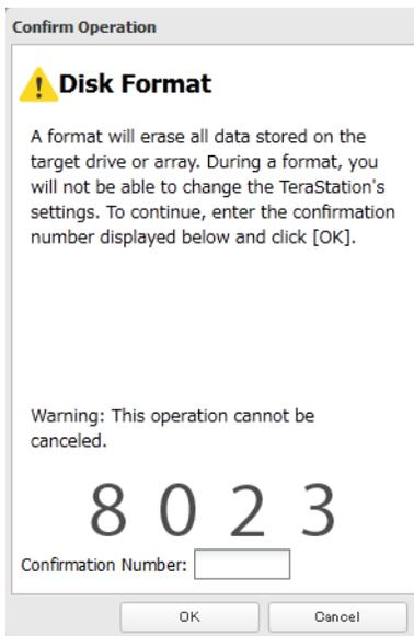
6 Depending on the size of your drive, the format may take several minutes or several hours to complete. “Formatting” will be displayed on the LCD display until the format is complete.
