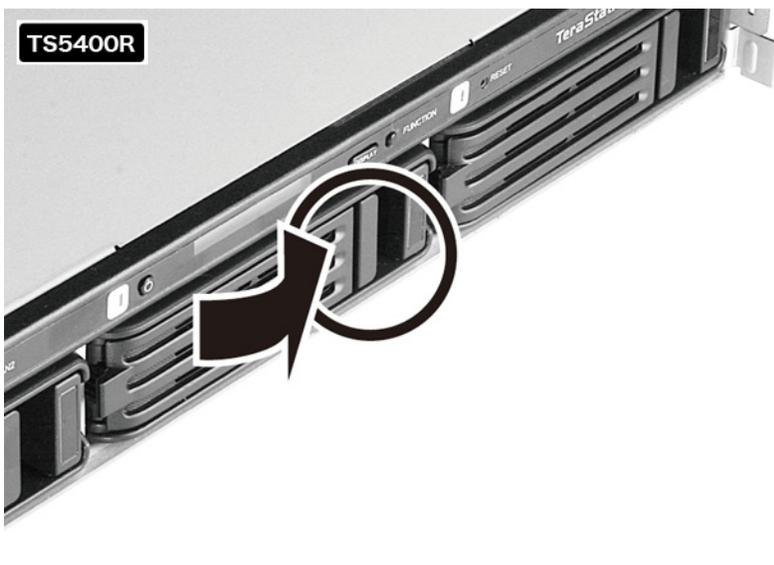
**6** When the replacement hard drive is recognized, the status LED will flash red and the message “Press FuncSW I31 New Disk x ready” will be displayed on the LCD panel.
