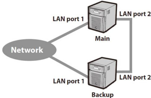
The main and backup TeraStations should be the same model and capacity. Use fixed IP addresses for both TeraStations. Because the IP address of the TeraStation designated as the backup cannot be changed, set its IP address before configuring failover.
