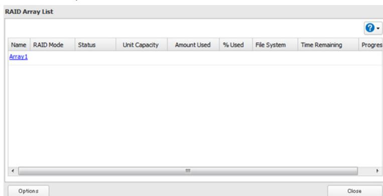
**Note:** If the “RAID Mode” field is blank, the array is already in JBOD. Proceed to step 7.
