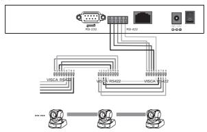
When using RS422 bus connection mode, the third pin (Ra) of the controller is connected to the TXD IN- of the camera, the fourth pin (Rb) of the controller is connected to the TXD IN+ of the camera, the first pin (Ta) of the controller is connected to the RXD IN- of the camera, and the second pin (Tb) of the controller is connected to the RXD IN-
