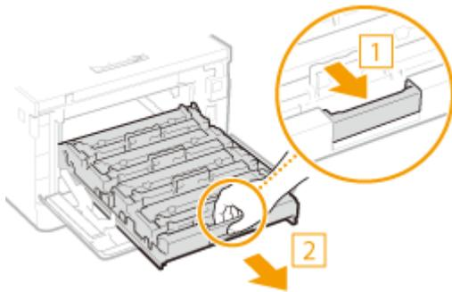
**3 Pull the target toner cartridge straight up and out of the machine.**
