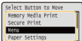
**3** Use ▲ / ▼ to move to the target position, and press **OK**.
