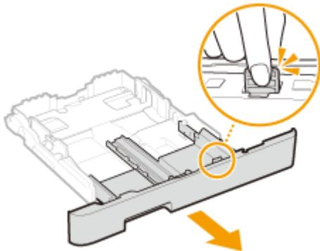
**3 Load the paper so that the edge of the paper stack is aligned against the paper guide on the front side of the paper drawer.**
