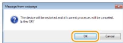
⇒ A restart process begins. Communication remains disconnected until the main unit has restarted.
