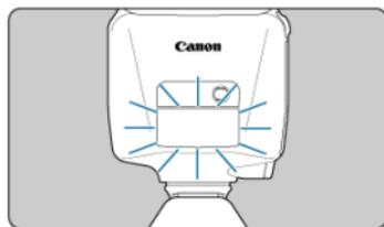
When it is difficult to autofocus on the subject in low-light or when contrast is low during viewfinder shooting, the infrared AF-assist beam built into the flash automatically flashes to help autofocus.
