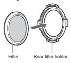
1 Attach the filter (\$\phi\$30.5mm) to the rear filter holder mounting thread.
