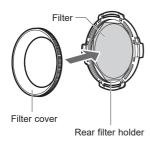
After attaching the filter to the rear filter holder, attach the filter cover to the rear filter holder mounting thread.
