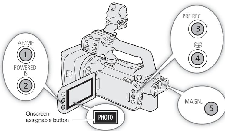
1 **Physical buttons:** Press the MENU button and, while holding it pressed down, press the assignable button whose function you wish to change.
