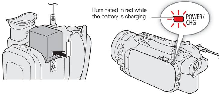
**4 When the POWER/CHG indicator goes out, the battery is fully charged.**
