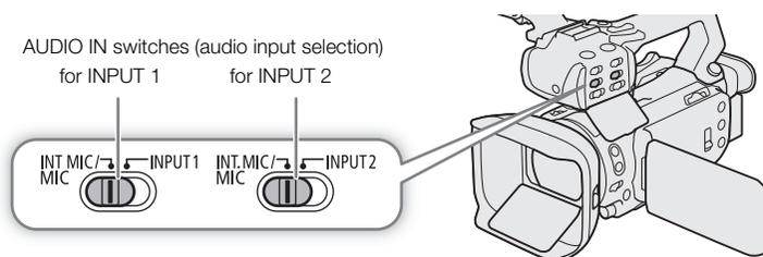
1 If the handle unit is connected to the camcorder, set the corresponding AUDIO IN switch to INT.MIC/MIC.
