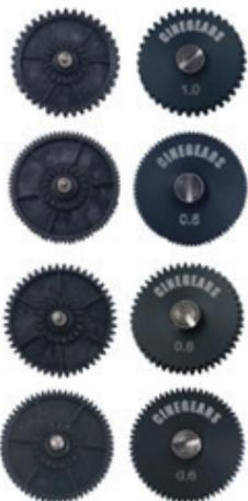
Cinegears 38mm Variety Pitch Replacement Gears are included, with the radius side of 38mm (original is 45mm), which can provide you with even smoother movement for small lenses. It also can work with different lenses with variety pitches. The pitch size includes: 1.0, 0.8, 0.6 and 0.5.
