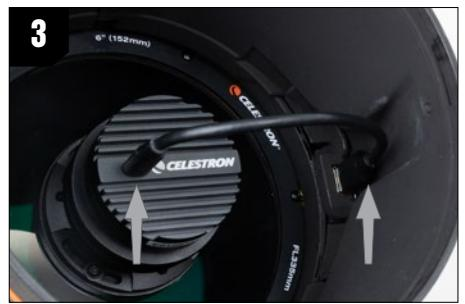
3. Plug the end of the USB camera cable into the port on the back of the camera.
