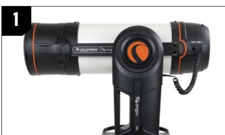
1. While supporting the Origin tube from underneath so it does not suddenly slide up or down, loosen the altitude clutch knob and carefully release the tube. If your Origin is properly balanced, the tube should remain in a horizontal position when the clutch knob is loosened. If it does, you can move on to the next section of this guide. If the tube moves up or down, proceed to step two.
