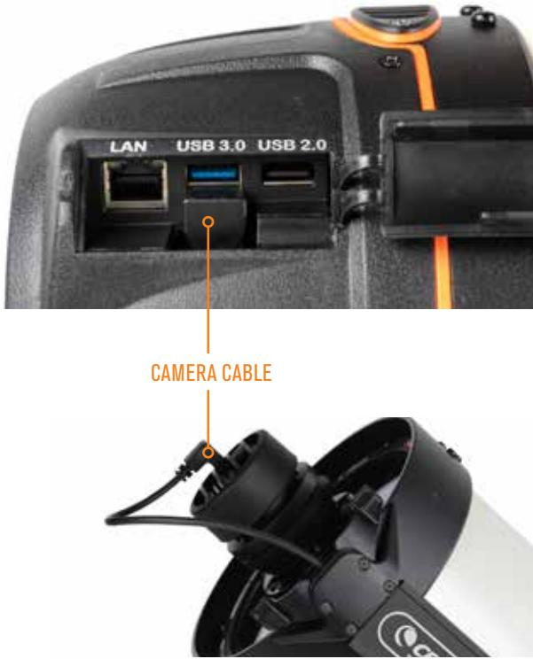
FIG 36: One end of the camera cable plugs into the camera. The other end plugs into one of Origin's USB ports.
