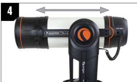
4. Gently slide the tube forward or backward a small amount to balance the scope and tighten the quick-release knob to secure it in place.
