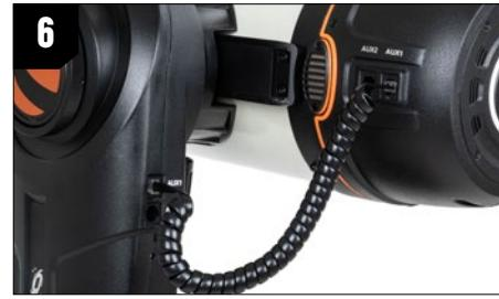
6. Plug the AUX cable from the port on the back of the Origin tube to the AUX port on the narrow side of the mount.
